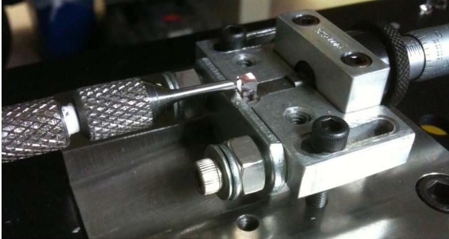
Figure 2. Test fixture set-up for sample fracture strength measurements (phosphate glass sample is shown).
